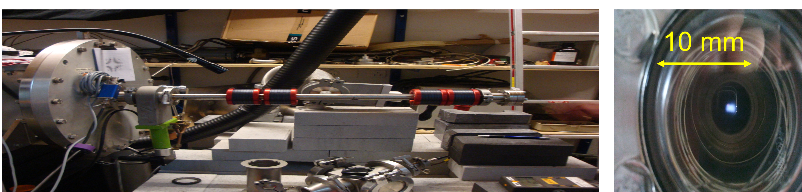
·Left: HEBT (length 55cm) consisting of four permanent magnet quadrupoles ·Right: focused beam made visible on glass scintillator (image size 2 \times 2 \text{ cm}^2 )
