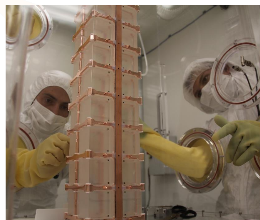
Assembly of the CUORE-0 tower
