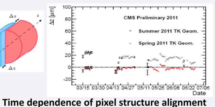
Alignment corrects for the shifts along z of the pixel
