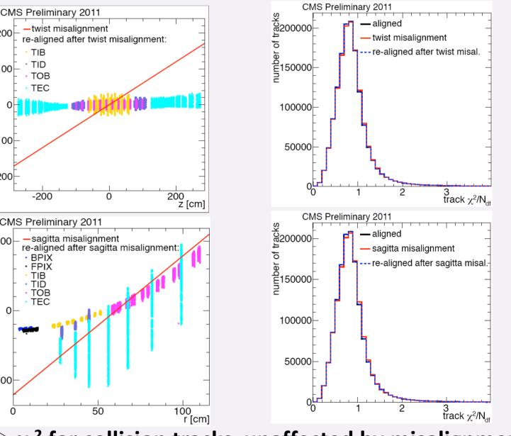
$\gg \chi^2$  for collision tracks unaffected by misalignment Applied twist misalignment eliminated after re-
