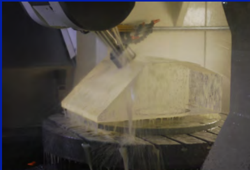
Machining more precise shape on NC machine:
