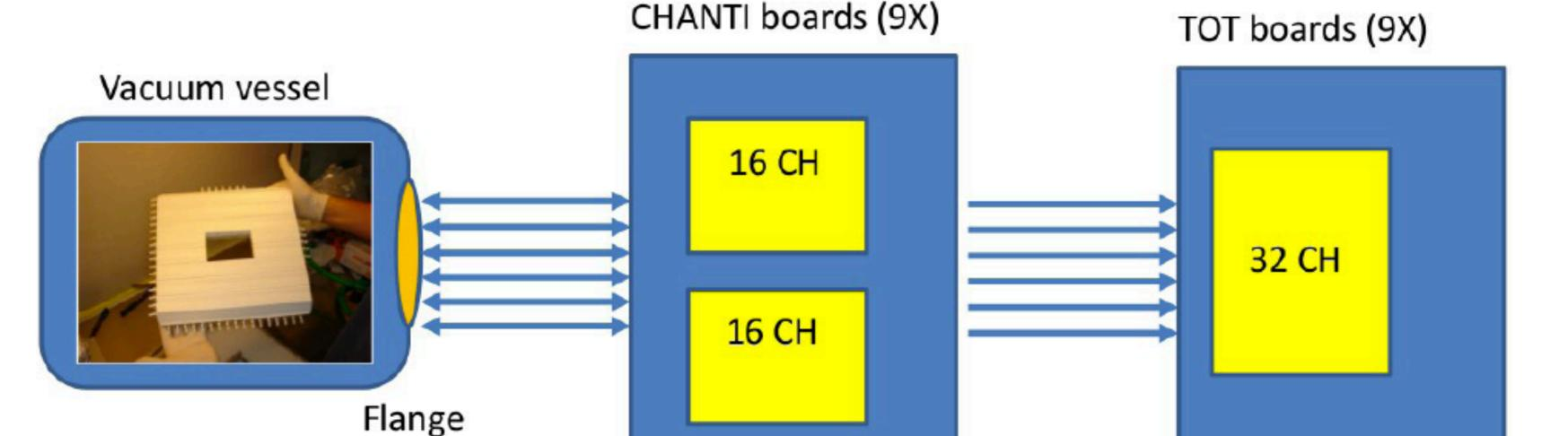
Preliminary tests have been done with cosmic rays using the first prototype station and a the FEE prototype board. External trigger has been used. About 120 photoelectrons have been collected for each layer. Time measurements, corrected for time slewing using TOT measurement, have shown a resolution of the order of 800 ps.
