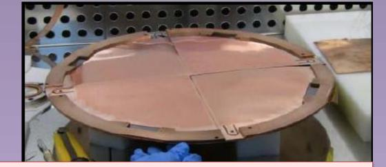
Largest area with µbulk technology Each sector radius = 14 cm 1252 pixels independently read 0.8 cm pixel 50 μm gap
