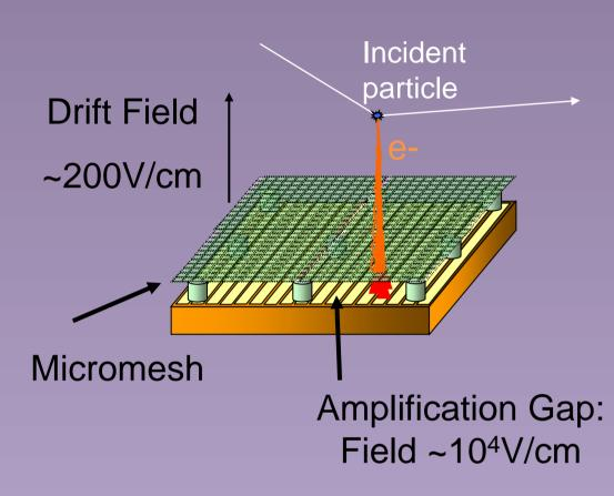
$\Box$  Robust and with gains >  $10^3$ □ Very good spatial resolution Tested up to 10 bar in Xe Under continuous development
