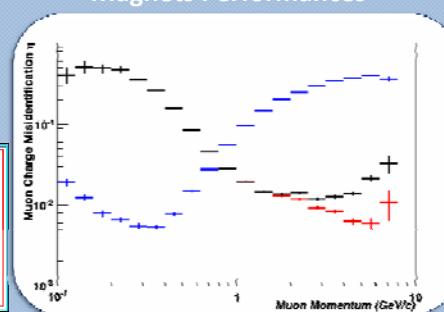
Blue markers: magnetic field on air, red (black) markers: magnetic field in iron with two (one) arms. Selection and reconstruction efficiency are included.
