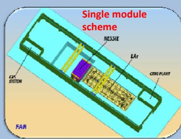
NESSIE is a modular detector formed by two (NEAR and FAR) Fe + Air spectrometers Placed downstream L-Ar\* detectors <sup>\*</sup>.
