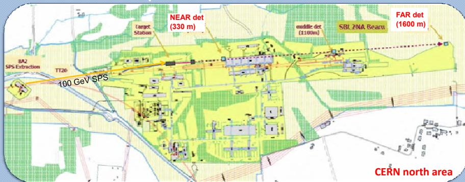
New SPS beam layout: - 100 GeV primary p fast extracted from SPS - on axis beam option
