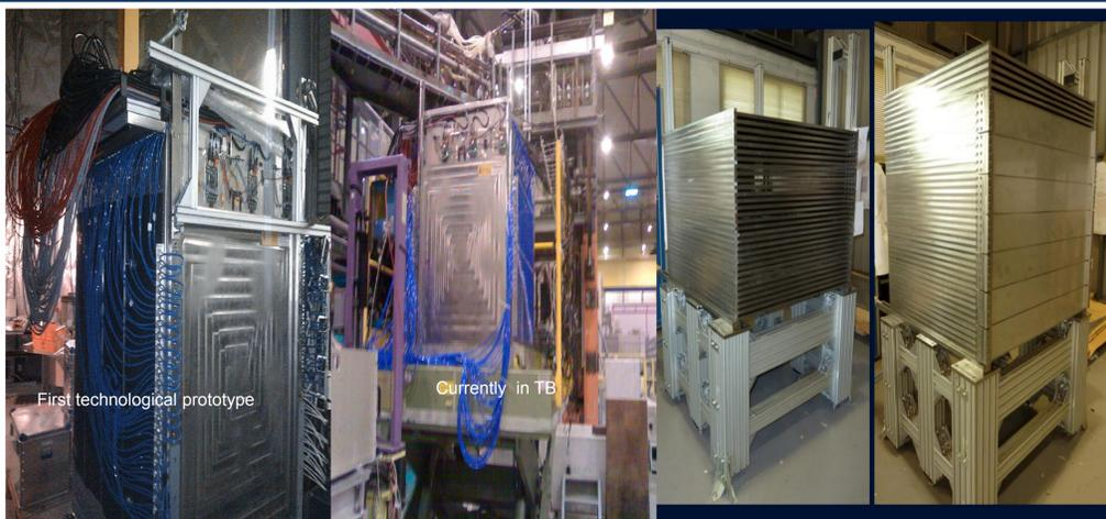
Construction of the SDHCAL prototype 460800 electronics channels And self-supporting mechanical structure 50 units (>6 λ<sub>r</sub>) working with power-pulsing
