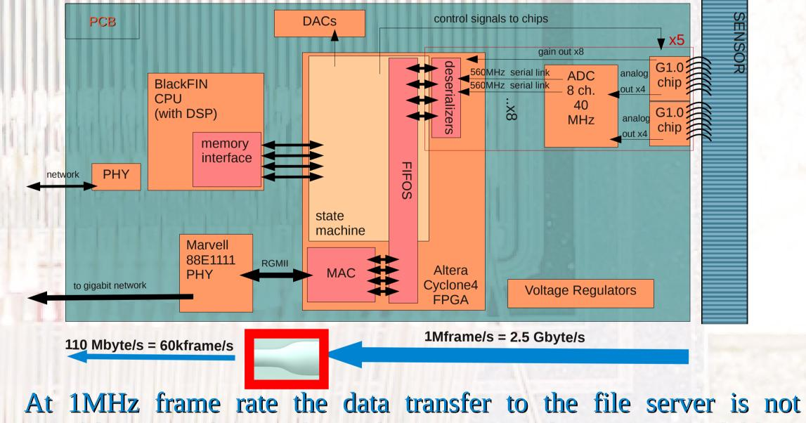
At 1MHz frame rate the data transfer to the file server is not possible. Depending on the application, two solutions are available.
