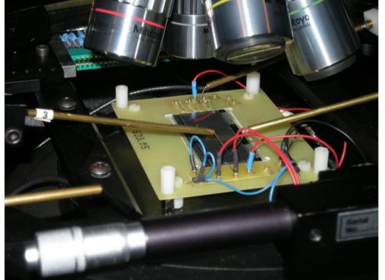
The strip capacitance in different pairing configurations has been measured on FBK-irst double-sided test sensors of BaBar-like design, but with parallel strips on p and n sides, 5.3 cm long, at 50 um pitch.
