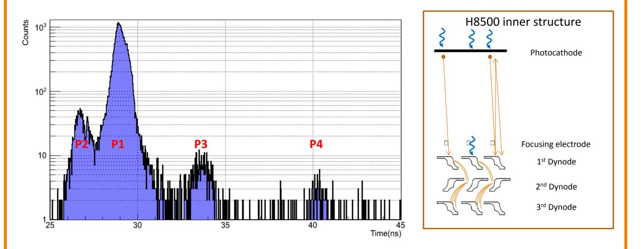
The time distribution is obtained by measuring the time between the laser pulse and the MaPMT detected signal.
