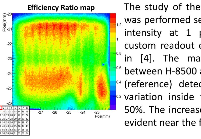
The study of the detection efficiency , was performed setting the laser beam intensity at 1 p.e. and using the custom readout electronics described in [4]. The map shows the ratio <sup>0.6</sup> between H-8500 and Photonis XP2020 <sup>0.4</sup> (reference) detection efficiency: the <sup>0.2</sup> variation inside the pixel is roughly 50%. The increase in efficiency is also evident near the focusing electrodes.
