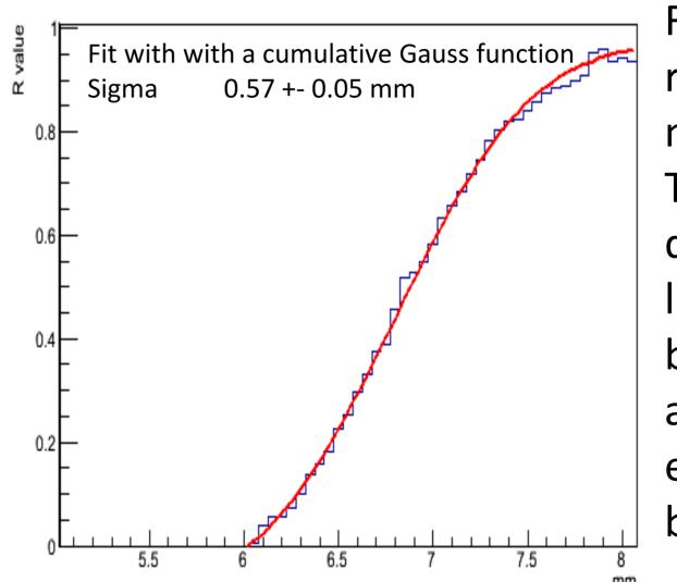
From the fit a charge sharing region of 600µm has been measured.
