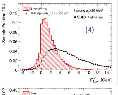
Examples of jet rejection variables: shower width in the electromagnetic and hadronic calorimeter weighted by the transverse energy of each calorimeter part (1), number of tracks in the isolation annulus (2), decay length significance of the secondary vertex for multi-prong tau candidates in the transverse plane (3), pileup corrected transverse energy of isolated clusters (4).
