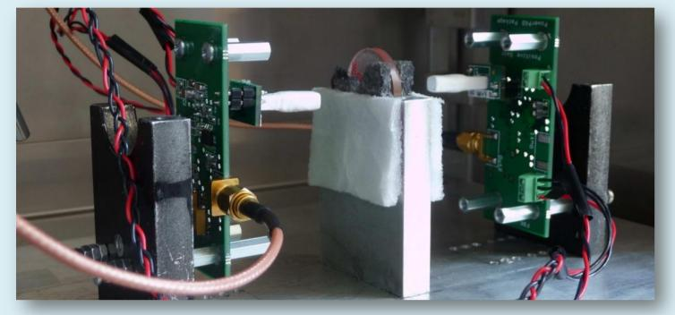
Optimized design to minimize parasitic. Amplifier's outputs are digitize by an oscilloscope.
