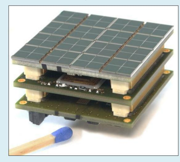
It composed of a SiPM (by FBK) tile, ASIC (PETA1 chip) tile and interface board. It proved to be MR compliant.
