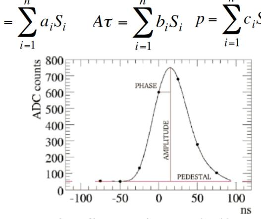
The iterative method is slower and more sensitive to noise fluctuation and pileup. The non iterative method allows to cope with the acquisition high rate, it is the design method, employed in online and also in the offline. It is crucial demonstrate that these methods give similar performances under suitable conditions.
