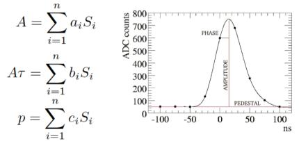
The iterative method is slower and more sensitive to noise fluctuation and pileup. The non iterative method allows to cope with the acquisition high rate, it is the design method, employed in online and also in the offline. It is crucial demonstrate that these methods give similar performances under suitable conditions.
