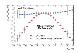
Variation in phase of pulses in the non iterative method causes an underestimation of amplitude. Deviation of the energy for small time variations within 1 bunch crossing can be corrected.
