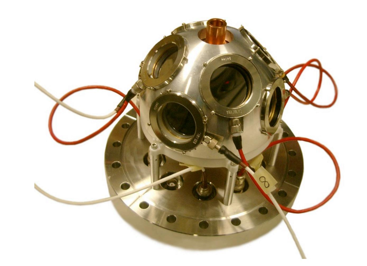
The chamber is comprised of two domes: The outer one is made from aluminum and houses the silicon detectors. The second, inner dome, is constructed from copper and directly connected to a cold trap. This is designed to reduce the deposition of carbon and nitrogen contaminants on the target surface. A bias of -300V is also applied to this dome in order to suppress the emission of secondary electrons. Eight 9 cm<sup>2</sup> silicon detectors are mounted to the
