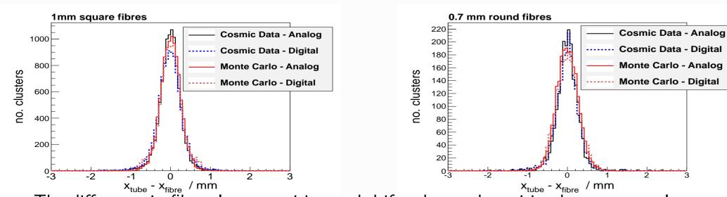
The difference in fibre cluster position and drift-tube track position have a normal distribution where the width is determined by the resolution of the fitted cosmic track from the drift tubes and the cluster position determined from hit-weighted (digital) or charge-weighted clusters (analog). The spectra shown above are for the optimal charge thresholds in a well-behaved part of the experimental setup.
