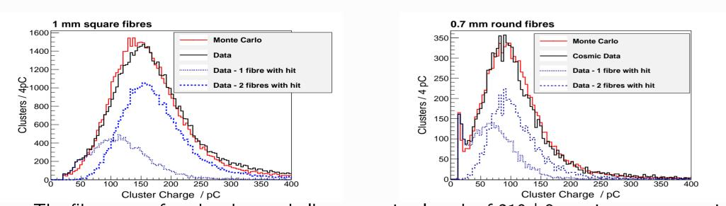
The combined resolutions of the drift tube track and fibre planes are shown above, with the resolutions extracted from the Monte Carlo truth information also shown. The cosmic data and Monte Carlo data agree well in both fibre plane tests. However, the drift tubes exhibits poor resolution in 3 regions along the edges of the tubes, as well is higher in the 0.7 mm tests due to lower statistics and residual miscalibrations.
