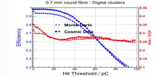
The effects of noise and crosstalk on the cosmic ray position resolution can be reduced by adjusting the charge threshold for which a channel is included in a charge-weighted (analog) or hit-weighted (digital) cluster. An increasingly large threshold eventually degrades the efficiency as well as the resolution.
