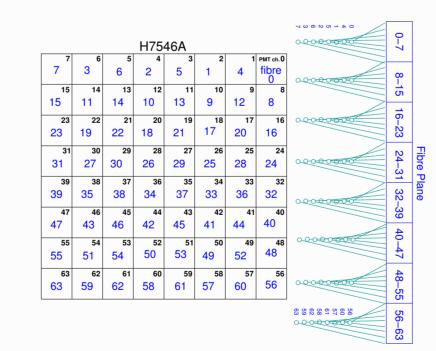
Electronic crosstalk and crosstalk from misalignment to the MA-PMT channels are managed by the fibre arrangement on the MA-PMT plane, and will not affect the track cluster width. However, there is some evidence for shared optical light between fibre channels, possibly due to localized emissions from the primary dye in the track fibre and absorption by the secondary dye in the adjacent fibre.
