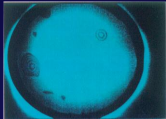
WAFER BONDING (mechanical stability) \text{Si-OH} + \text{HO-Si} \rightarrow \text{Si-O-Si} + \text{H}_2\text{O}
