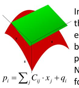
In each found road the parameters of the track candidates can be calculated exploiting linearized constraints between the hit positions and helix parameters. Naturally parallel approach, well suited for modern FPGAs
