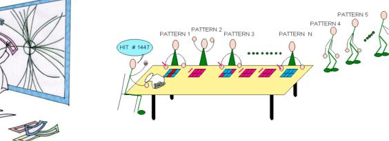
The pattern matching can be parallelized with the use of special CAM-like memories, using parallel match-lines that compare the incoming hits with a list of physical pre-calculated patterns, using a coarser resolution
