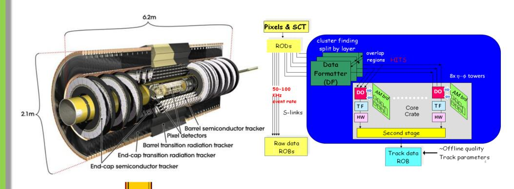
The Fast Tracker processor is designed to read all the silicon layers of the Inner Detector (ID)
