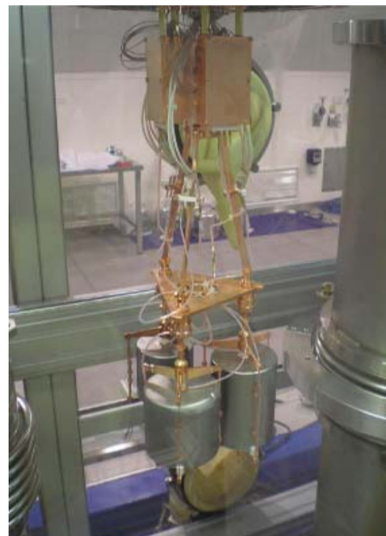
Fig. 3: The three-string arm inside the GERDA glove box, holding three Ge detectors during the set-up phase.
