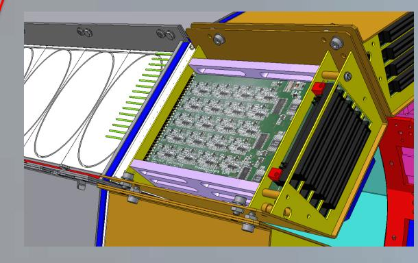
Each fiber readout by a single 1.2 diameter circular SiPM.
