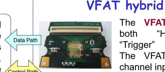
The **VFAT** produces both "Hits" and "Trigger" information. The VFAT has 128 channel inputs.
