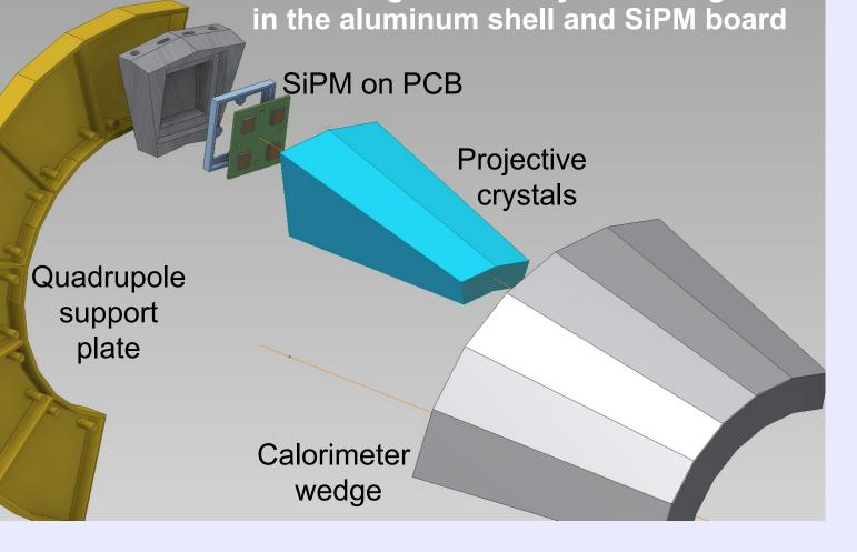
CAD drawings for the crystal arrangement
