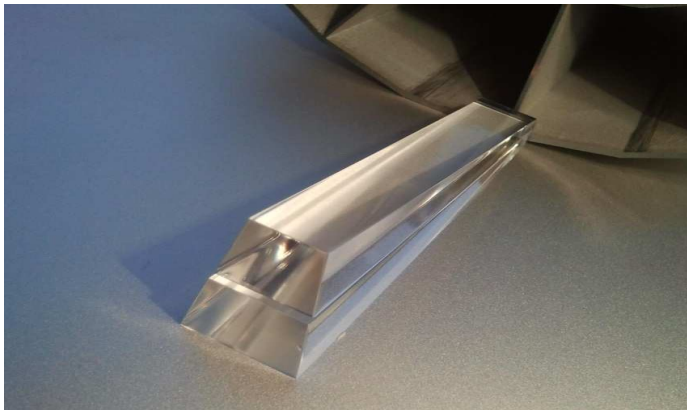
First two crystals under test ( ^{22}\text{Na} source + PM readout) 10% energy resolution @ 511 keV
