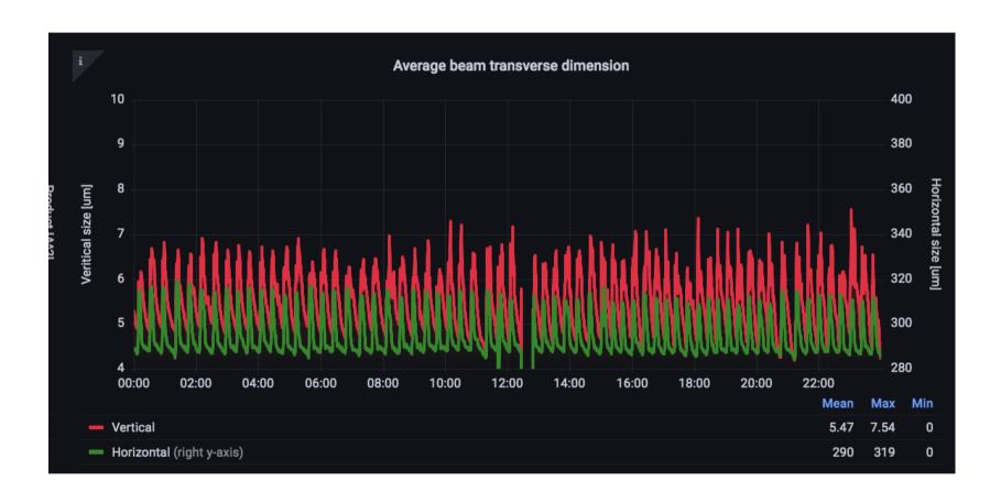
Oct 24<sup>th</sup> run Convoluted transverse dimension of colliding beams are under control
