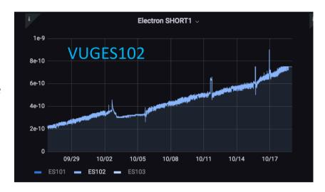
Electron beam was clearly affected by ion trapping although there was no clear evidence of vacuum issues.
