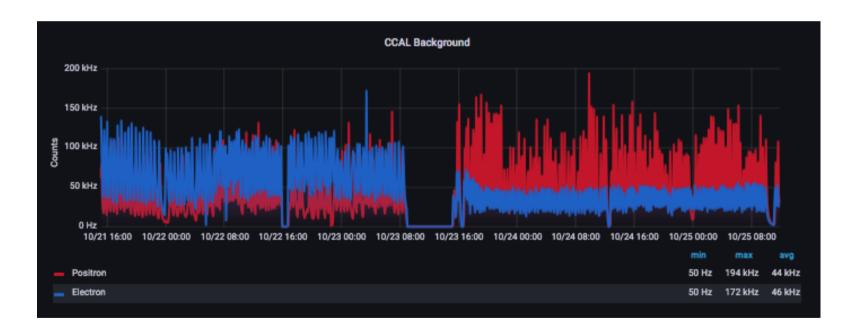
After fixing the small vacuum leak ion trapping effects disappeared.
