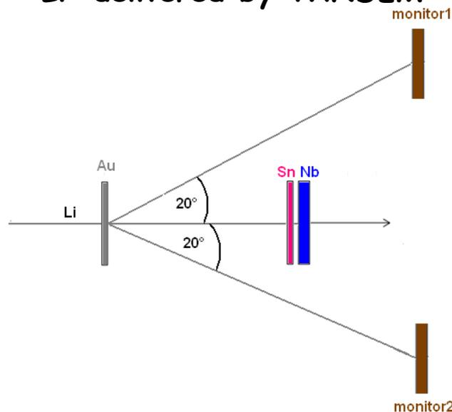
${}^{93}\text{Nb}$  catchers are used in order to stop the residues emerging from the target
