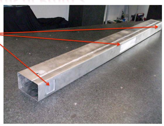
1 additional flange for gas tightness still to be machined
