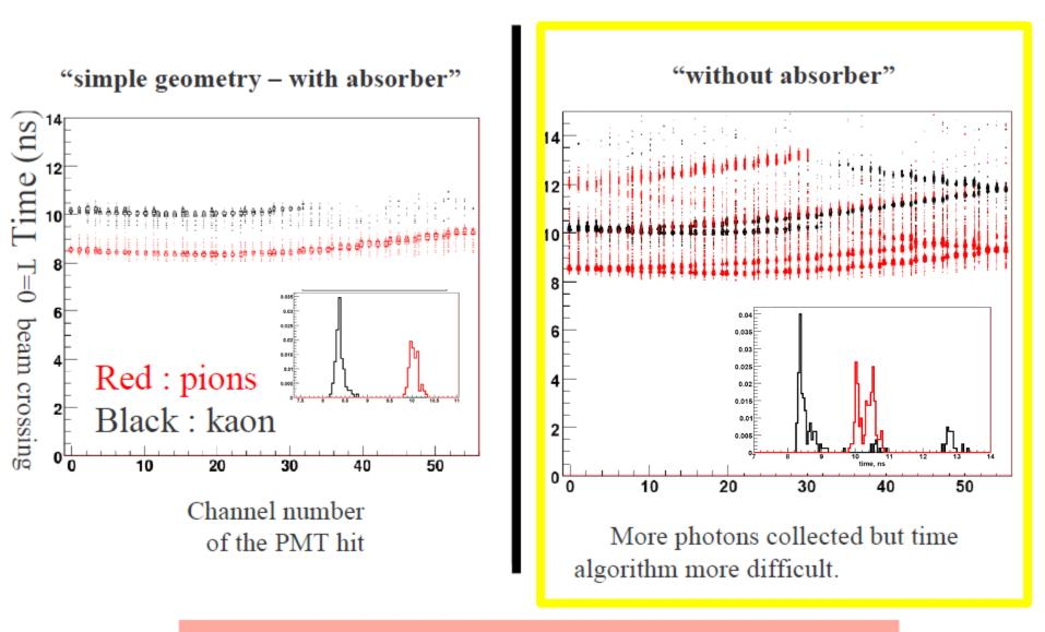
FTOF is a 2D device because it measures time vs position
