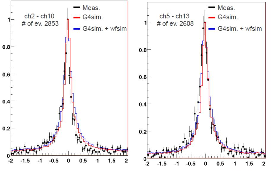
Average time resolution calculated using this type of time differences is ~100ps = 70ps/channel.
