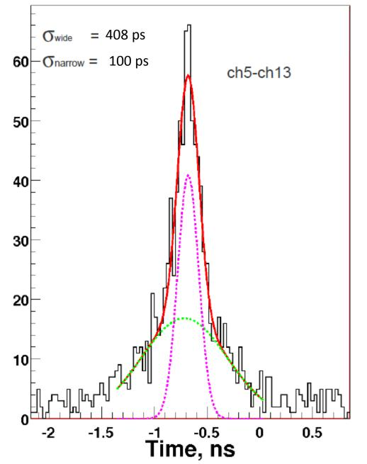
Example for time difference expected In the simulation between two channels
