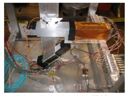
• Two quartz bars connected to one Photonis MCP-PMT (8x8 channels, stepped face, 10 micron holes).
