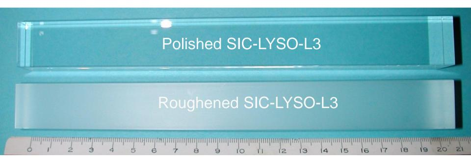
1st: lapped to Ra = 0.5 by using 11  $\mu$ m Al<sub>2</sub>O<sub>3</sub> powder for 10 min with 2.5 kg weight. 2nd: lapped to Ra = 0.3 by using 6.5  $\mu$ m SiC powder for 3 min with 1.5 kg weight.
