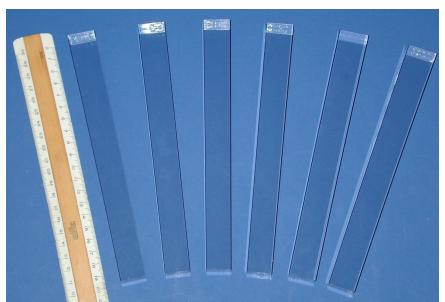
Φ60 x 250 mm ingots are cut to two 20 cm long crystals for a SuperB beam test at CERN last Fall.
