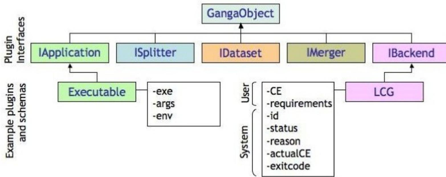
“Plugins for different types of application, backend, dataset, splitter and merger inherit from interface classes, which have a common base class. Schemas for the Executable application and for the LCG backend are shown as examples.”
