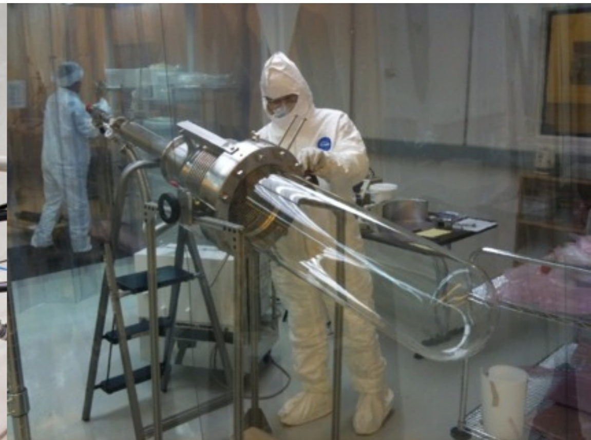
Fused silica inner vessel for 60-kg chamber. High purity construction techniques are used to reduce contamination by environmental radioisotopes
