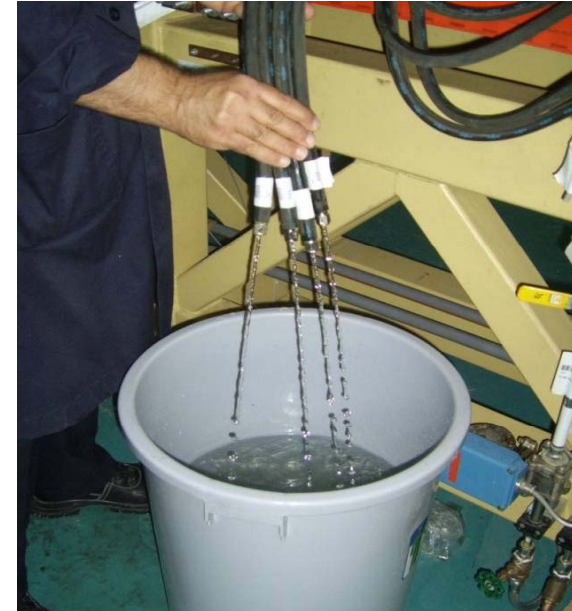
Water Magnet Cleaning
