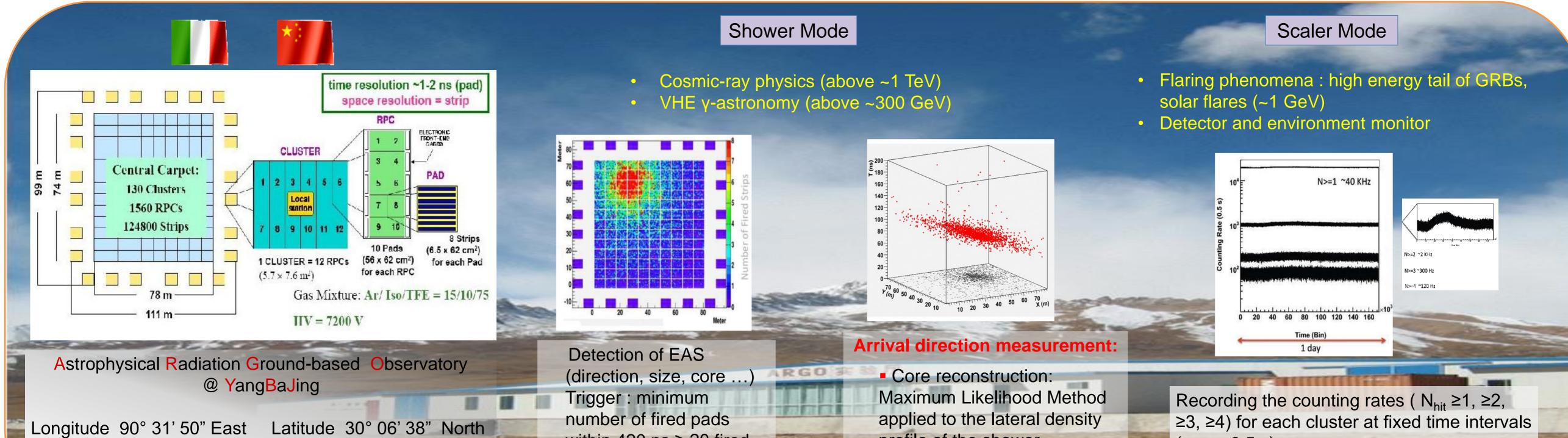
4300 m a.s.l., Total area =  $6700 \text{ m}^2$ Full coverage (92% active surface ) =  $5600 \text{ m}^2$  within 420 ns  $\ge$  20 fired pads on the central carpet: rate ~3.6 kHz
