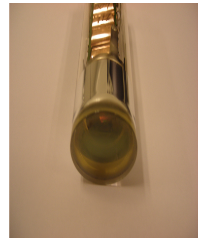
Photonis XP3102 borosilicate glass bialkali cathode, WLS applied
