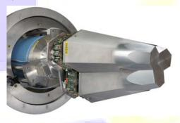
The concept of gamma-ray tracking relies upon the possibility of operating bulk germanium crystals in position-sensitive mode, so as to be able to locate the individual interaction points and determine the path taken by the gamma rays inside the spectrometer. The development phase of this detection technique is close to completion and the first gamma-ray tracking modules are already part of the AGATA Demonstrator array at INFN, Laboratori Nazionali di Legnaro.
