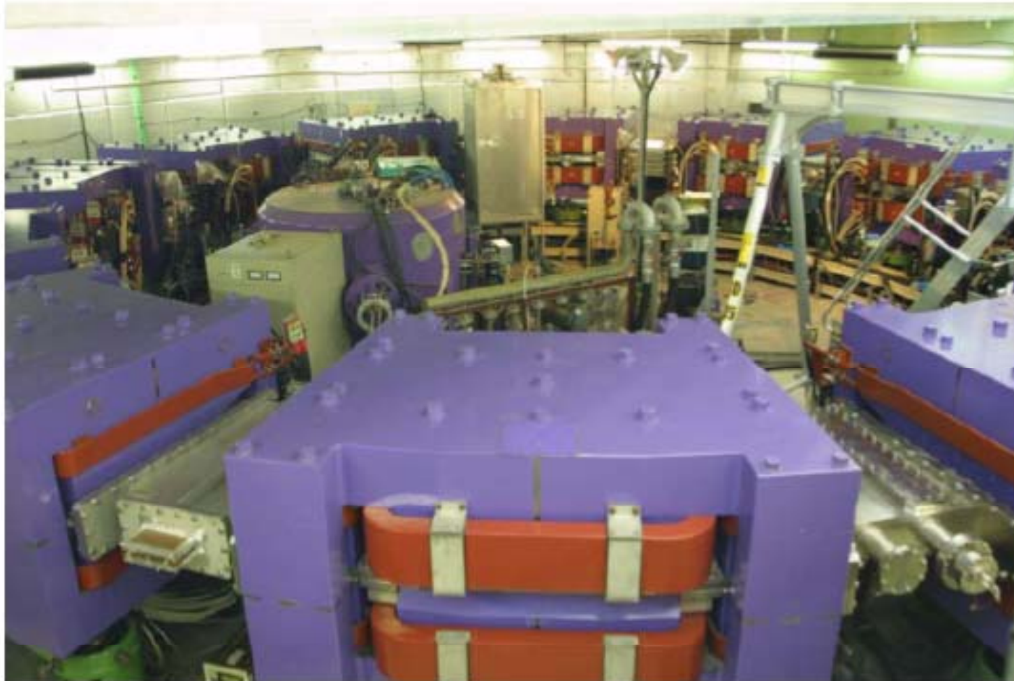
Fig. 7. The first proton therapy radial sector 150 MeV S-FFAG, built and commissioned at KEK in 2003.
