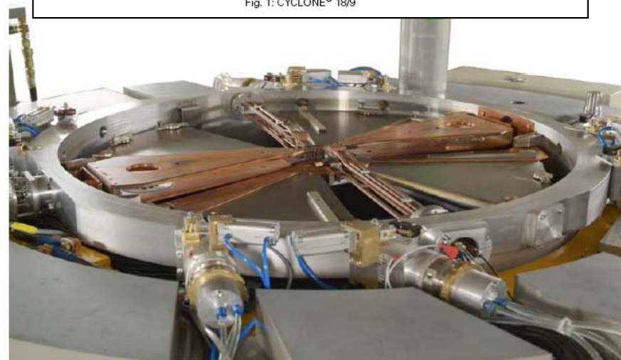
Fig. 2: CYCLONE® 18/9 median plane showing the Dees and 4-sector poles
