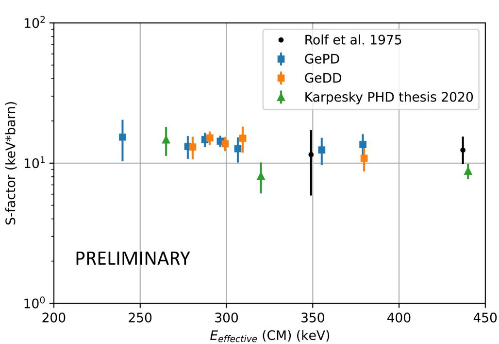
Since the direct capture takes place **throughout the whole chamber**, where different proton beam energies are achieved, we have associated to our S-factor values an effective energy. **E**<sub>effective</sub> represents the beam energy in the center of mass at the position where **half of the experimental yield is** obtained.
