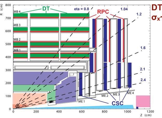
DT 2 Super Layers ( $\phi\theta\phi$ ) for first 3 stations  $\sigma_x\sim200~\mu m^2~\phi$  Super Layers in last station
