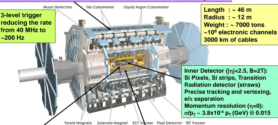
**EM calorimeter: Pb-LAr Accordion**
