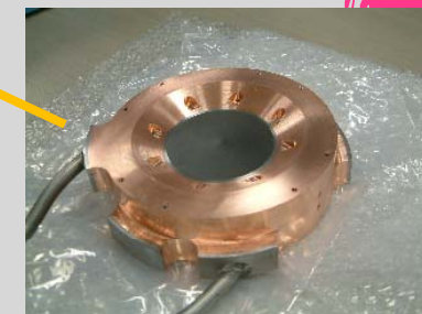
Graphite target with water cooling
