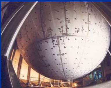
Stainless Steel Sphere ( d = 13.7 \text{ m} , Volume = 1340 \text{ m}^3 )
