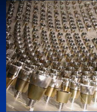
2212 8" ETL 9351 PMTs mounted inside the SSS
