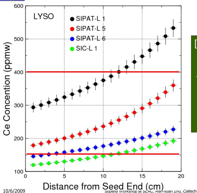
[Ce] in both SIPAT and SIC samples needs to be further optimized.
