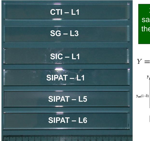
25 x 25 x 200 mm samples measured for their L.R.U. and fit to a linear function
