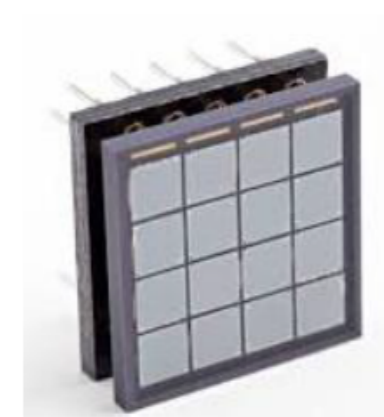
SiPM matrix directly coupled to end of detector
