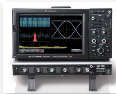
WaveRunner 625Zi 2.5 GHz, 20 GS/s, 4ch, 16 Mpts/Ch DSO with 12.1" WXGA Color Display, 50 ohm and 1 Mohm Input, 40 GS/s and 32 Mpts/Ch in interleaved mode.
