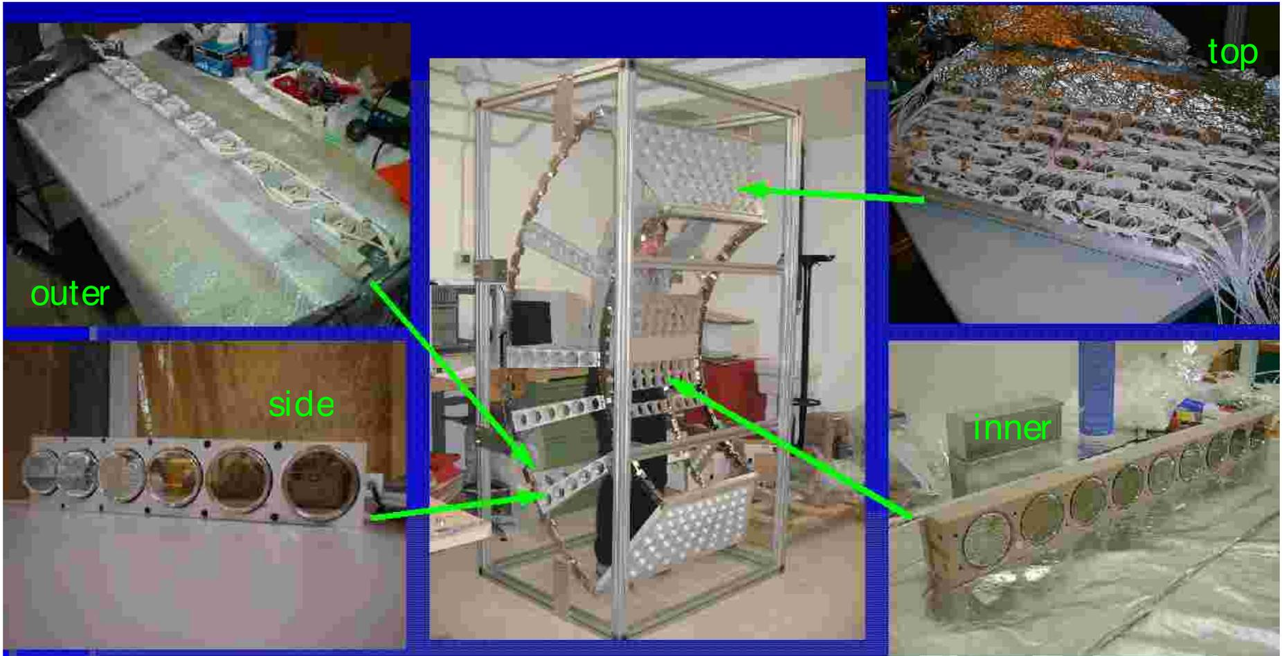
PMTs are installed into PMT holders
