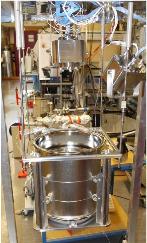
HV tests of ~30cm scale geometries
