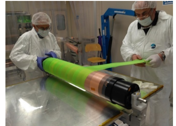
gluing with vaccum bag technique
