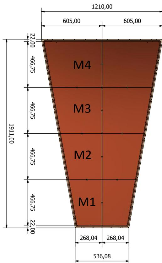
**A very large  $\mu$ -RWELL** with the dimensions close to the GE2/1 chamber is going to be realized at LNF, in collaboration with INFN-BA and INFN-BO with M4 operating detectors.
