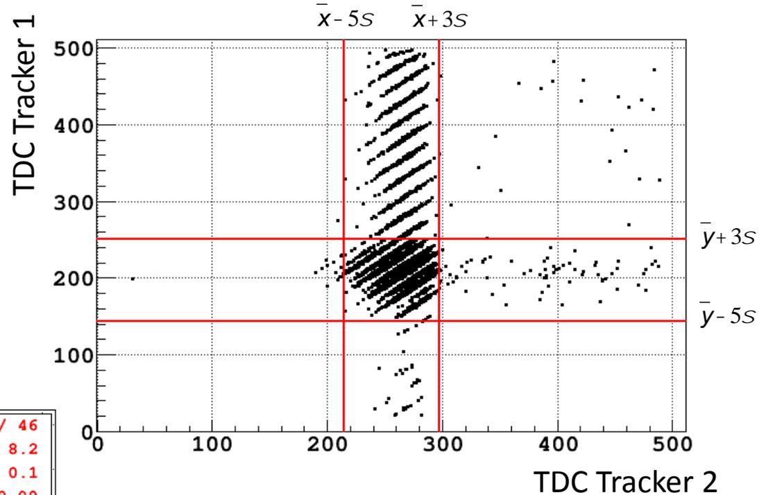
The TDC distribution is then fitted with a simple gaussian and the sigma is then **deconvoluted** by the contribution of the VFAT.
