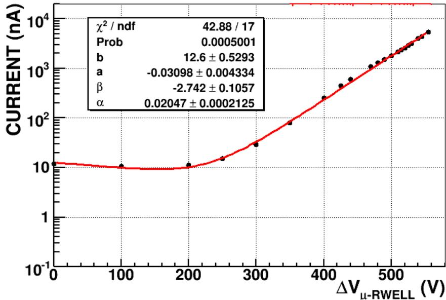
$I(g=4000) \sim 5 \text{ nA/cm}^2$  corresponding to an equivalent mip rate of  $\sim 60\text{-}90 \text{ kHz/cm}^2$  evaluated on sectors #3
