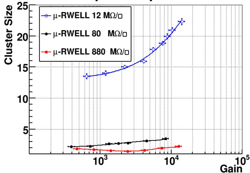
At low resistivity the spread of the charge (cluster size) on the readout strips increases, thus requiring a higher gain to reach the full detector efficiency.
