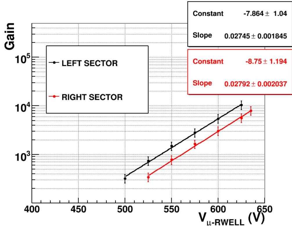
A shift of  $\sim 25$  V has been measured between the two sectors probably due to the **different** geometry of the amplification stage **(to be confirmed with microscope check – left/right asymmetry)**
