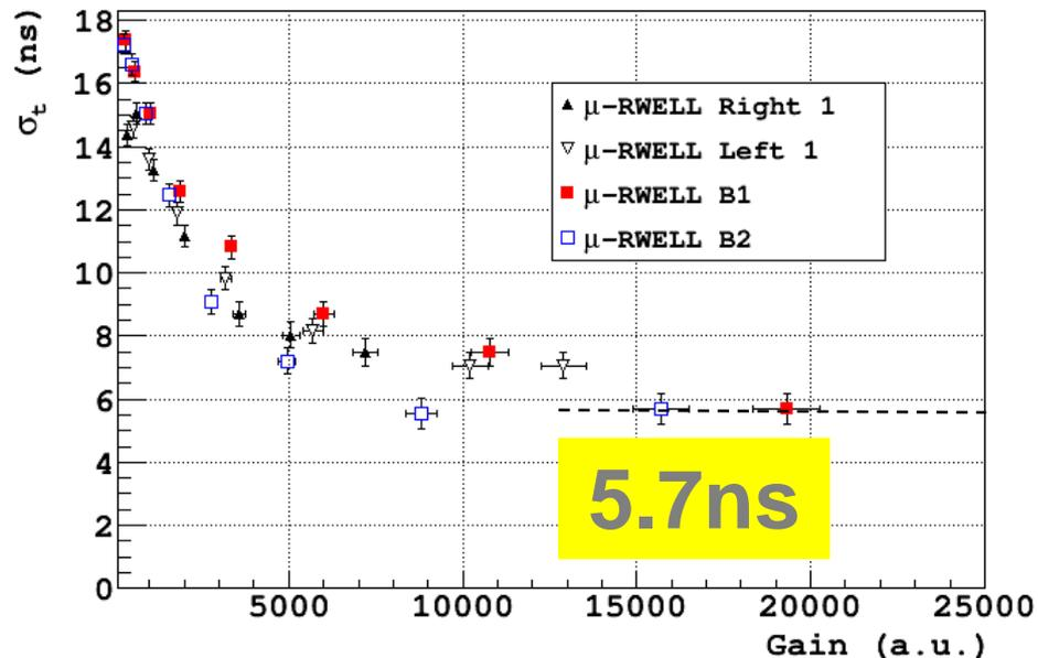
To be compared with a measurement done with GEM by LHCb-LNF in 2004 (LHCb) giving a  $\sigma_t = 4.5$  ns with VTX chip [1].
