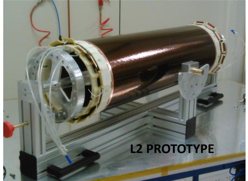
The BESIII-Italy collaboration is realizing three cylindrical GEMs to replace the inner part of the Drift Chamber.
