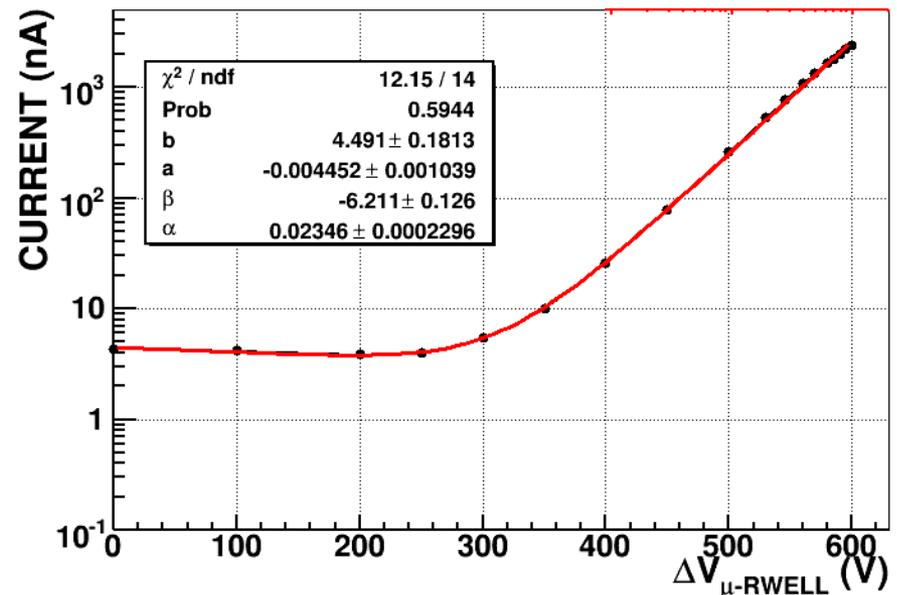
$I(g=4000) \sim 10 \text{ nA/cm}^2$  corresponding to an equivalent mip rate of  $\sim 250 \text{ kHz/cm}^2$
