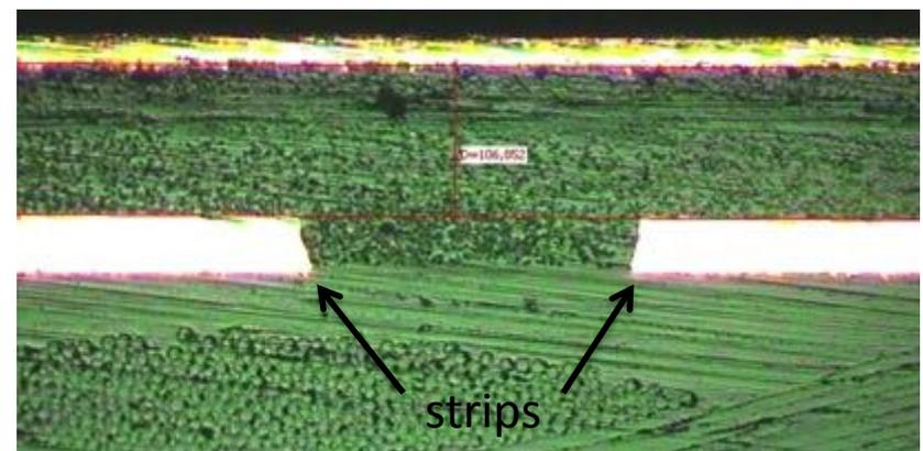
Metallographic cross sections: on the left we have an example with one pre-preg layer (50  $\mu\text{m}$ ), on the right with two pre-preg layers (100  $\mu\text{m}$ )
