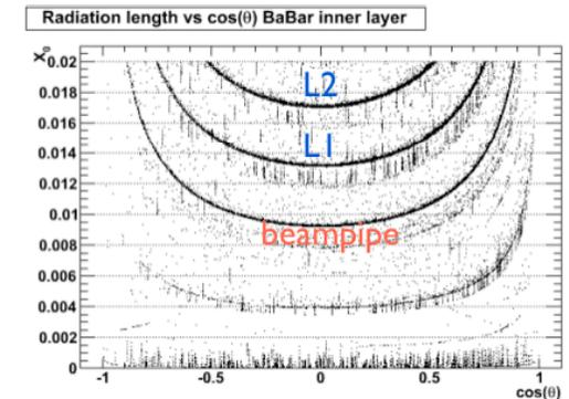
Total amount of L0 material is  $\sim 1.36\% X_0$  considering overlap of passive material. Relative amount of material for Al bus and support-cooling requires small adjustments.
